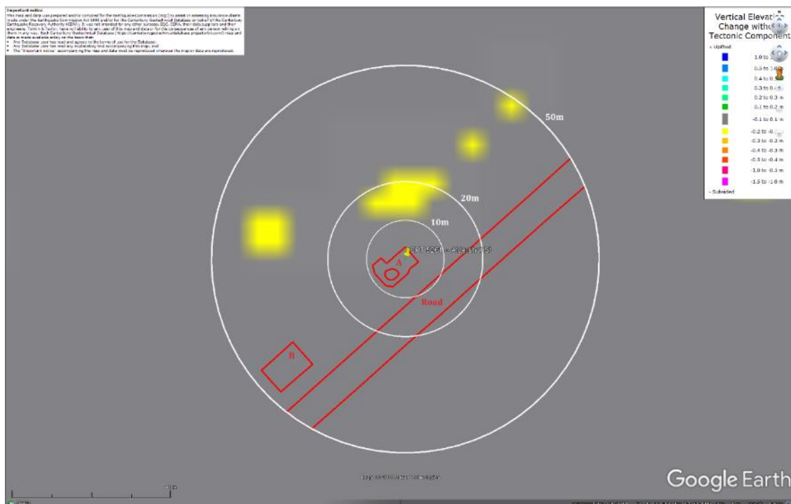
Figure 33: Ground surface subsidence without tectonic component for June 2011 Earthquake according to the LiDAR DEM.
